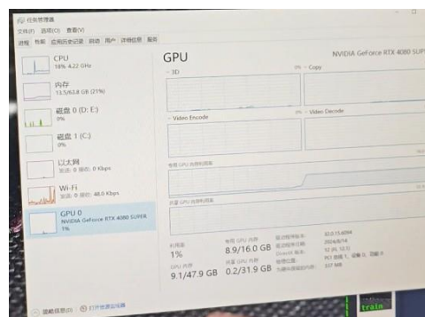
Fig. 4 The configuration of computer hardware for running the AI inspection system program
